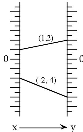
Two in-out lines are shown in the above diagram. Each one is labeled with a number pair. The first number in the pair is the input, and the second number is the output.
